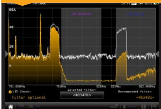
It analyses the impact of the LTE signal on the DTT channels, and detects whether the use of filters is required. Furthermore, it allows spectrum simulation upon the introduction of the LTE filter recommended by the meter itself. A list of filters is displayed for the user to choose the one that best fits his/her requirements.
