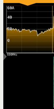
Signal graphic displays signal levels turning on the time axis. Short signal interference observation would be captured in the spectrum.
