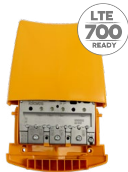
▲ High-gain Mast Amplifier 120 x 130 x 40 mm
