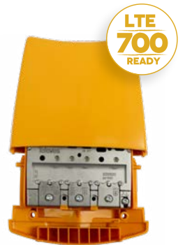
Terrestrial Mast Amplifier 120 x 130 x 40 mm
