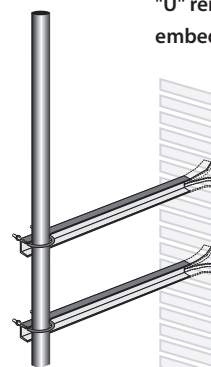
"U" reinforced bracket for embedding mounting
