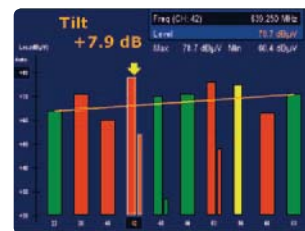
TILT You can analyze the possible imbalances between the existent channels in a TV network.
