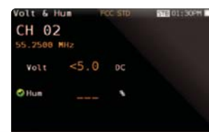
VOLTIMETER AND HUM VOLTAGE AND NOISE POWER PRESENT IN THE CABLE NETWORK
