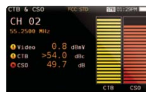
CSO & CTB DETAILED PARAMETERS OF THE ANALOGUE SIGNAL
