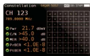
CONSTITUTION SCREEN ANALYZES IN DETAIL THE QAM SIGNAL
