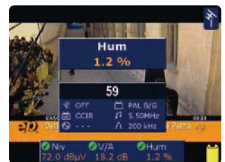
CTB/CSO & HUM Numerical measurements (dB) to identify problems within a CATV network generated by active devices.
