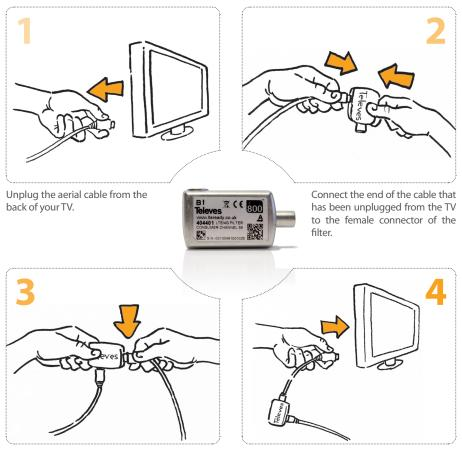
Connect the female connector on the cable lead to the male connector on the filter.
