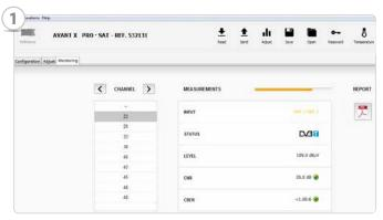
1. After the installation is completed, we connect to the Avant X Pro unit via the **Asuite application** (Android/Windows/Mac) and access the monitoring screen.
