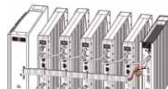
Powering with 15 Vdc from the PSU
