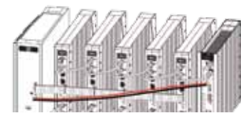
Powering with 24 Vdc from the PSU
