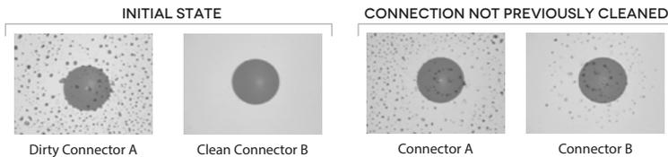
a clean connector and a dirty one, and how a dirty connector can contaminate a clean one. The entire installation could even become contaminated if it is connected at various points that were not cleaned beforehand ■
