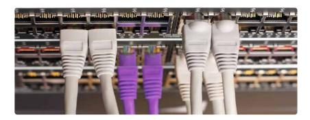
Yes, it is technically possible to mix devices of different categories as long as they are mechanically compatible, but it will be the lowest category element that limits the speed and bandwidth of the entire network. For this reason it is not recommended if you want to have the network working at maximum level of capacity and performance.
