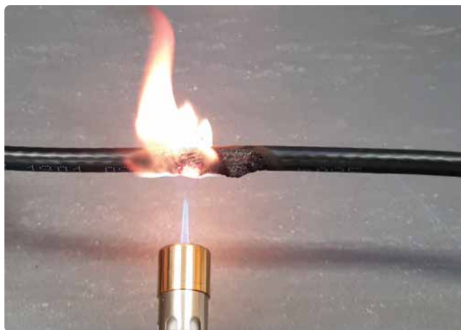
Fire test with a PVC cable, where we see that it is more flammable and emits smoke.
