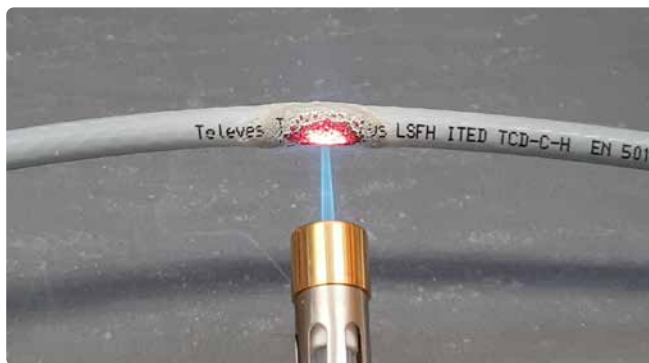
Fire test with an LSFH cable, where we see that it does not emit smoke and minimizes the spread of flames.
