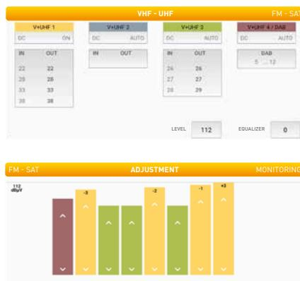
On the main screen, you can also set the output level and apply equalization (tilt) to the output if required.
