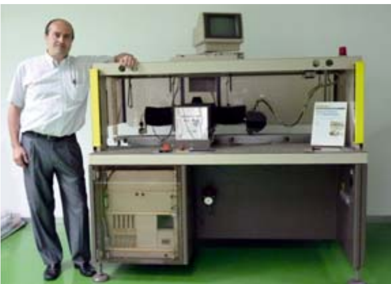
Jorge Montero Gabarro (Manufacturing Manager Televes/Spain) showing the first SMT machine MS 72 installed 1983
