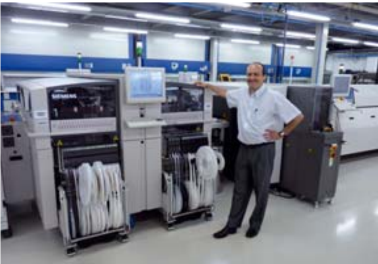
The new SMT production line at Televés/Spain for bare die and classic SMD placement consisting of Siplace Chip Assembly machine and SX2
